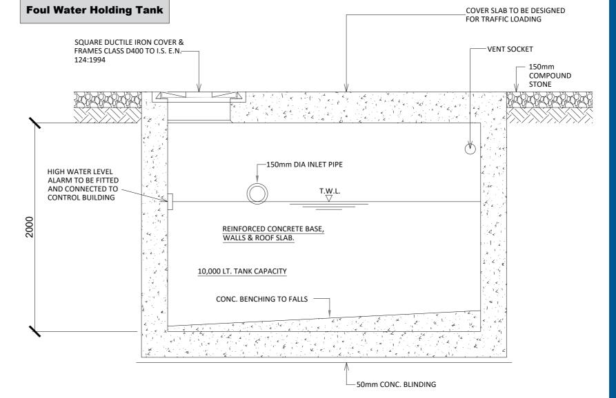
Foul Water Holding Tank - Elevation
