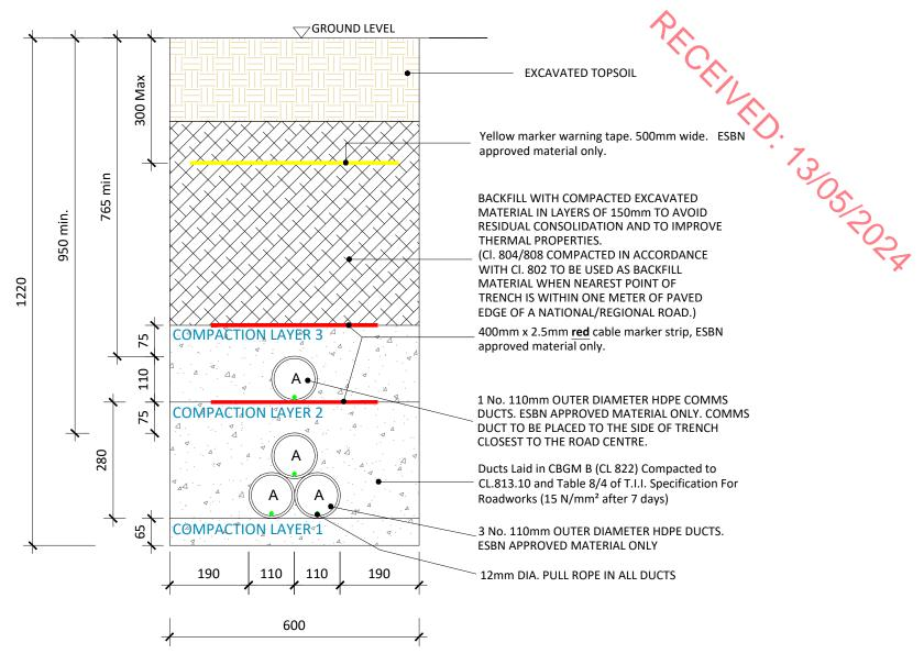
A =110mm:Outer diameter HDPE ESB Approved Duct, SDR=17.6;
