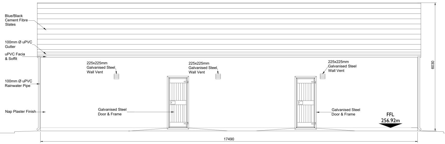
Front Elevation (Section A-A)
