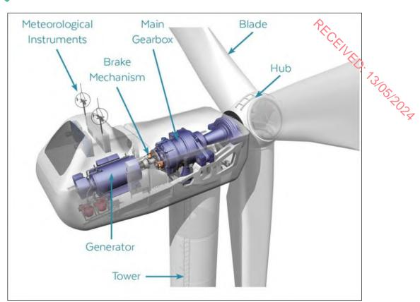
Figure 4-5 Turbine nacelle and-5 hub components
